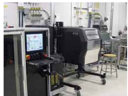
Testing to Improve Durability: The Center for Sustainable Mobility is partnering with Delphi to conduct tests of their solid oxide fuel cell system to further develop the product durability and reliability, as well as develop cost-effective manufacturing processes of solid oxide fuel cells.
