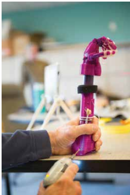
Assembly Required: After the prosthetic device is printed, Meetze assembles Lusie's arm with a natural grip posture.
