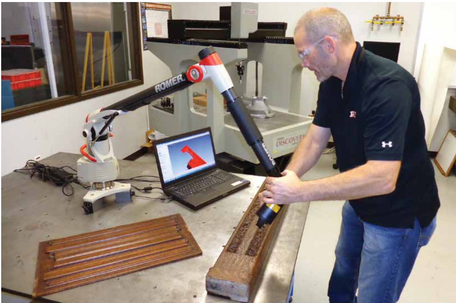
Digital Reproduction: Using a 3D laser scanner, Mike Bradley, a materials lab technician at RIT, creates a digital reproduction of a hand-carved pillar from St. Patrick's Cathedral in New York City.
