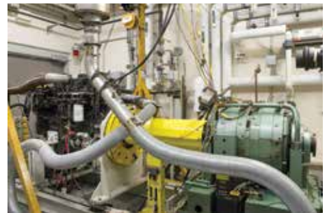
Stress Test Engines: Dynamometers are part of RIT's Vehicle Dynamics testbed. Companies work with RIT researchers to evaluate new fuels or vehicle technologies on engine and chassis dynos.
