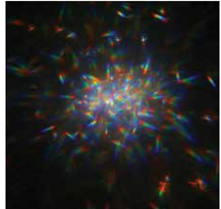
Smart Dust Technology: This image shows white light reflected off of a glitter mirror onto a camera sensor. Researchers tested this as part of a low-cost solution for space telescope mirrors.
