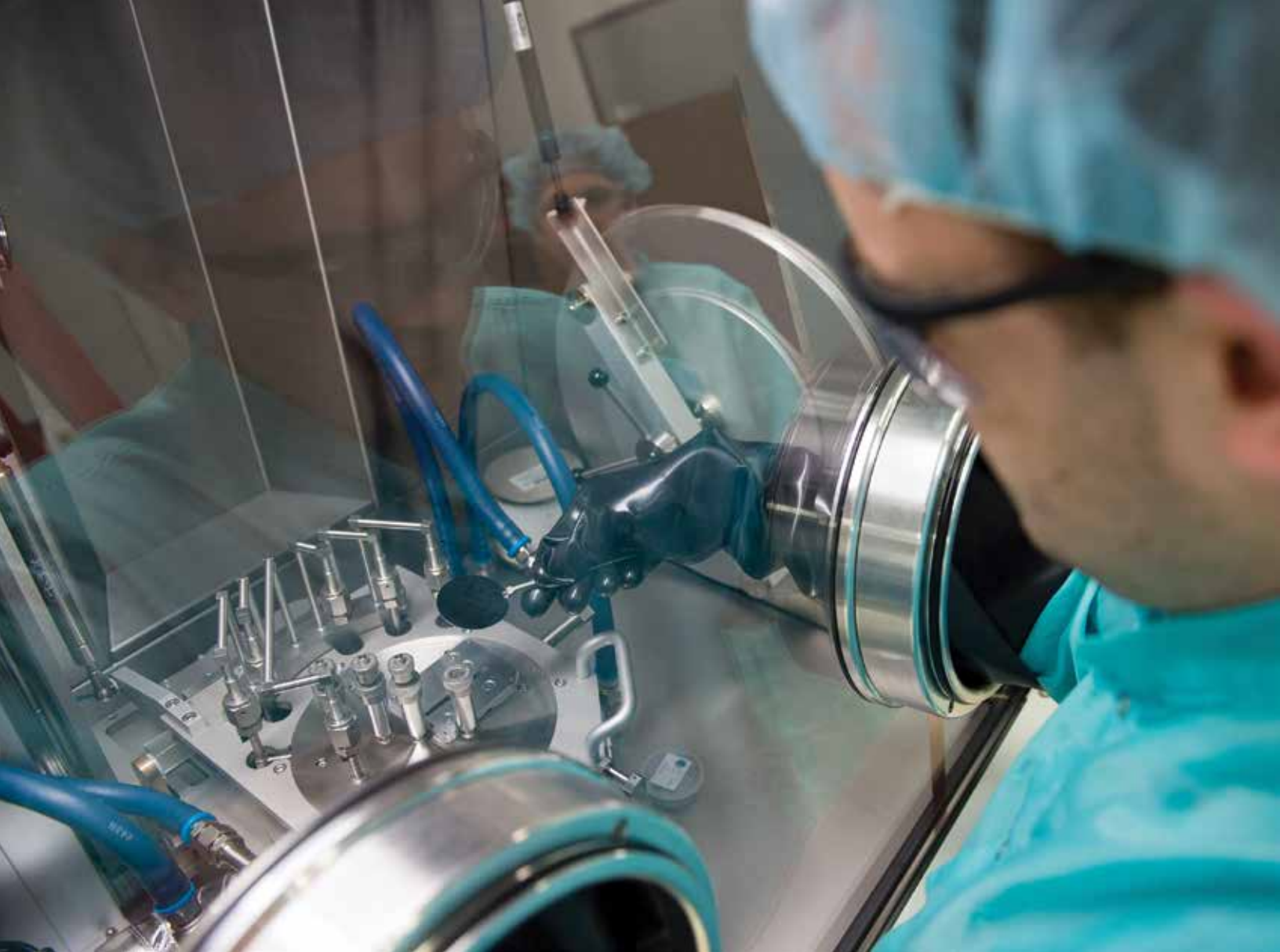
Growth Process: Michael Slocum, an RIT research scientist and recent graduate of the microsystems engineering Ph.D. program, prepares to load a new wafer in the MOVPE system.
