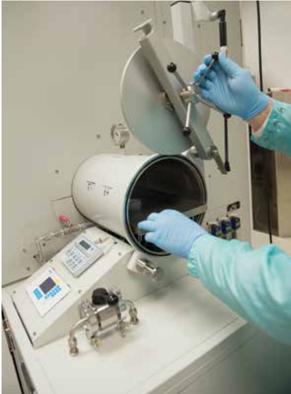
MOVPE Chamber: The chamber is enclosed in a nitrogen-filled ultra-clean glovebox to prevent contamination. After growth of new materials, the wafers are removed from the glovebox using a specially designed load-lock system.
