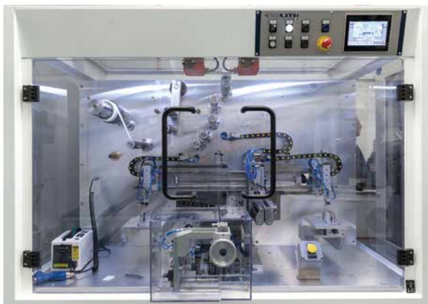
State-of-the-Art Equipment: The semi-automated Z-Fold machine uses robotic arms to stack cathodes and anodes.
