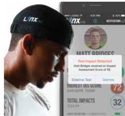
Wearable Head Technology: The Linx Impact Assessment System (IAS) uses a sensor that fits into a custom headband or skullcap. Using the companion mobile app, parents, coaches, and athletic trainers can monitor the force and frequency of impact to an athlete’s head.
