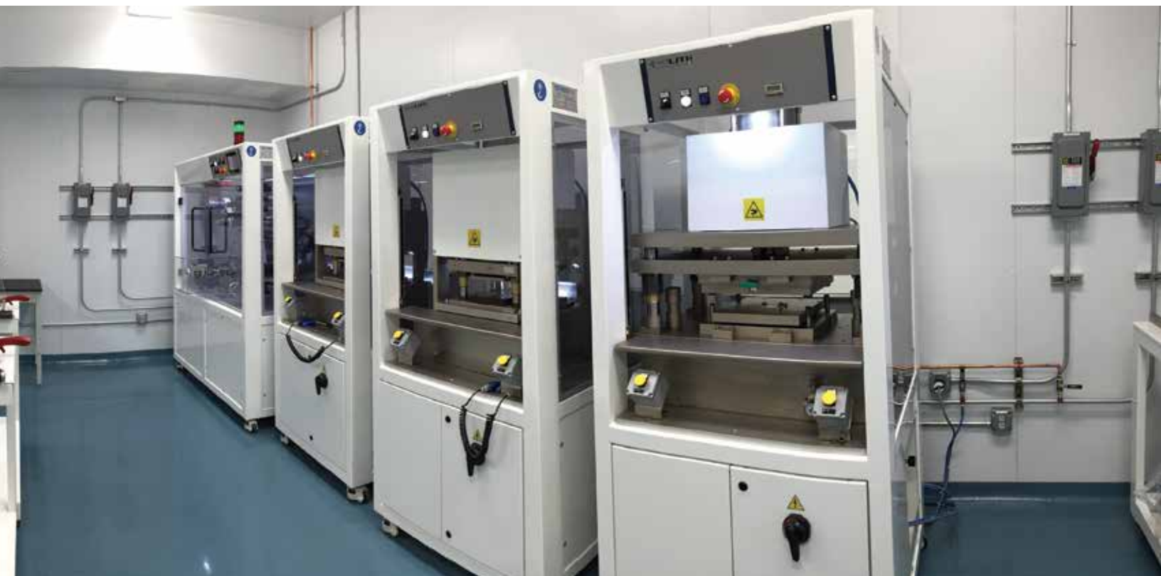
Prototyping Capabilities: Panoramic view of the prototyping portion of the dryroom, which is equipped with individual stations necessary to create a pouch cell.
