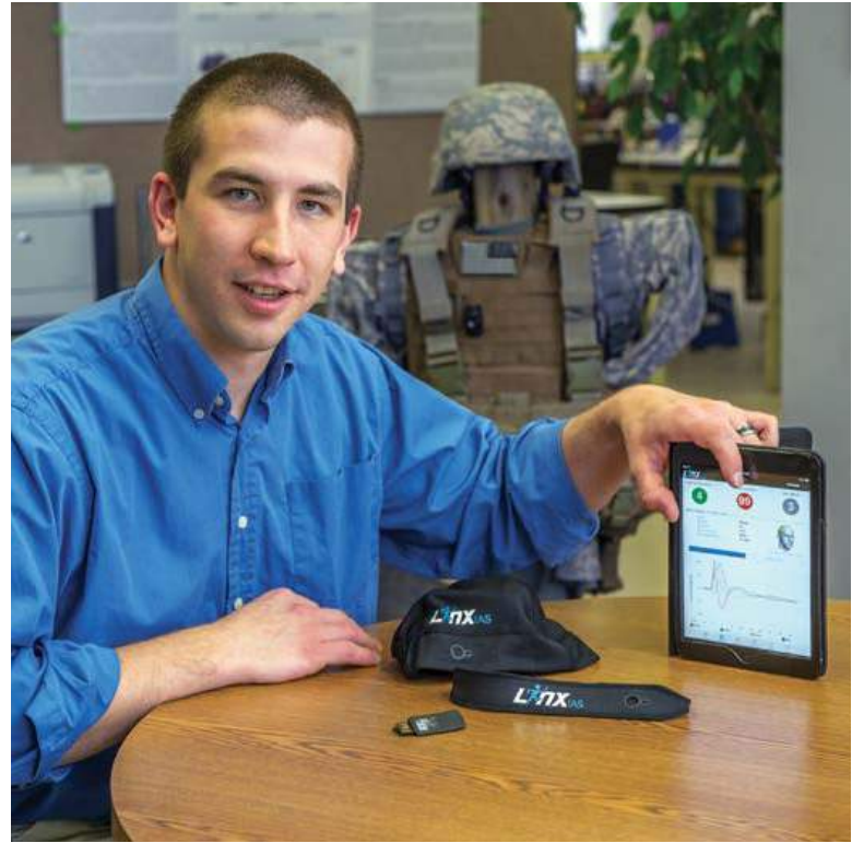
Monitoring Head Injuries on the Field: David Gillette '14 (electrical engineering) shows off BlackBox Biometric's sports impact-monitoring system, Linx IAS.
