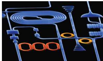
Integrated Photonic Chip: Scanning electron microscope image of an integrated photonic chip with many types of silicon waveguide devices and ring resonator filters (colored).
