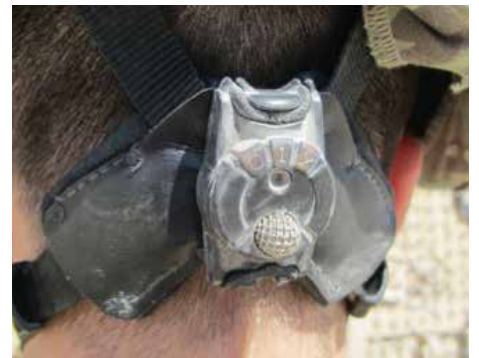
Protecting Soldiers in the Field: The blast gauge was originally developed through a research project funded by DARPA to better analyze the impact of concussive forces and reduce injury to soldiers. Above, a soldier wears a head-mounted blast gauge while on patrol.
