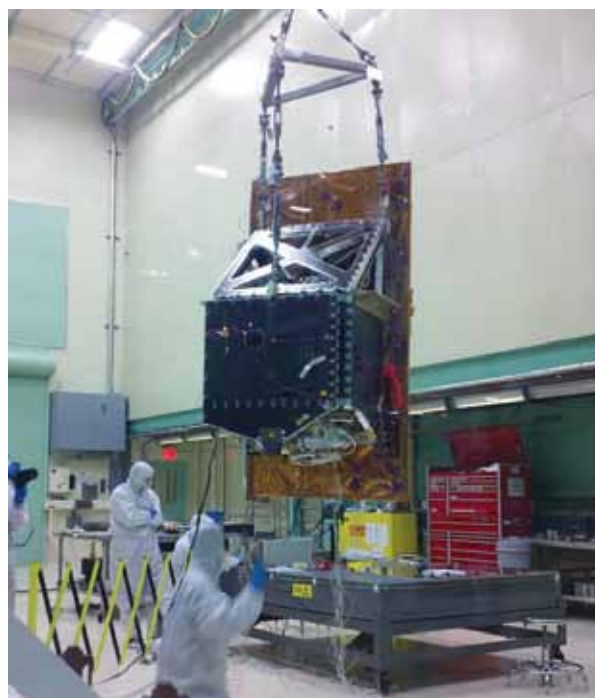
Creating the Next-Generation Imaging Satellite: The team is working with the Goddard Space Flight Center to design key instrumentation for Landsat 8, which is scheduled to launch in 2012. This includes testing of the Thermal Infrared Sensor, pictured above, which utilizes novel detector technology that has never been tested in space. Photo provided by Matthew Montero, Goddard Space Flight Center.
