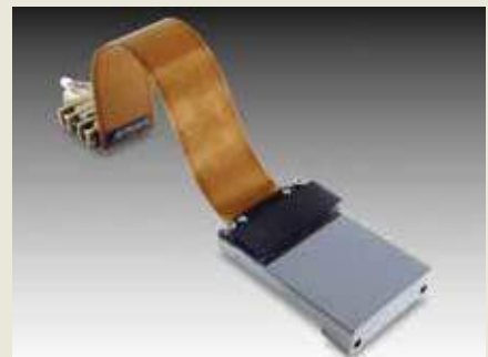
The Raytheon VIRGO 2Kx2K infrared detector is much like the ones RIT and Raytheon will design, fabricate, and test.
