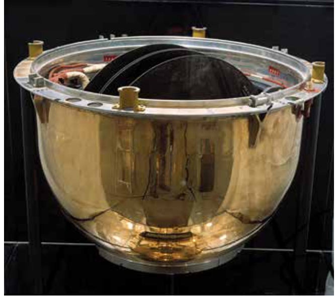
Reconnaissance satellite: The Corona KH-4B Camera and Discoverer XIII Film Return Capsule. It was the most advanced camera system used in Project Corona, the world's first photoreconnaissance satellite program. Photo by Eric Long, National Air and Space Museum
