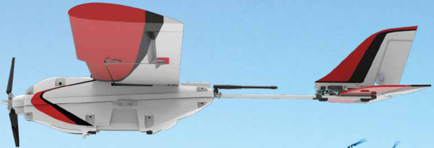
PrecisionHawk Lancaster: PrecisionHawk of Toronto, Ontario, has provided RIT with its Lancaster fixed-wing aircraft capable of lifting imaging sensors to altitudes up to 400 feet for up to 45 minutes.
