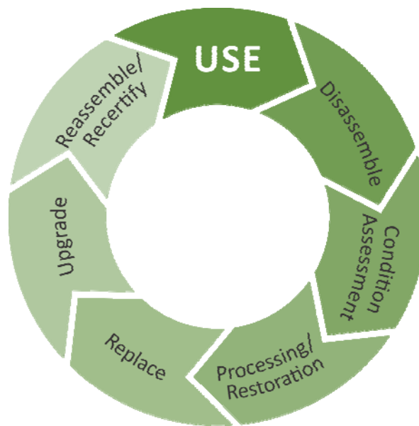
Figure 2. Remanufacturing Process Flow
