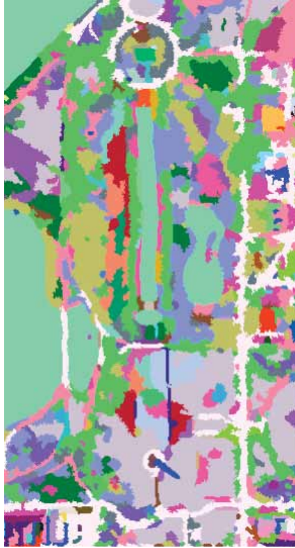
Segmentation for Remote Sensing: Image segmentation can be used as a pre-processing step for many remote sensing applications. A hyperspectral image of Washington, D.C., is segmented so that each color represents a region, distinguishing landmarks, roadways, buildings, waterways, and other characteristics.
