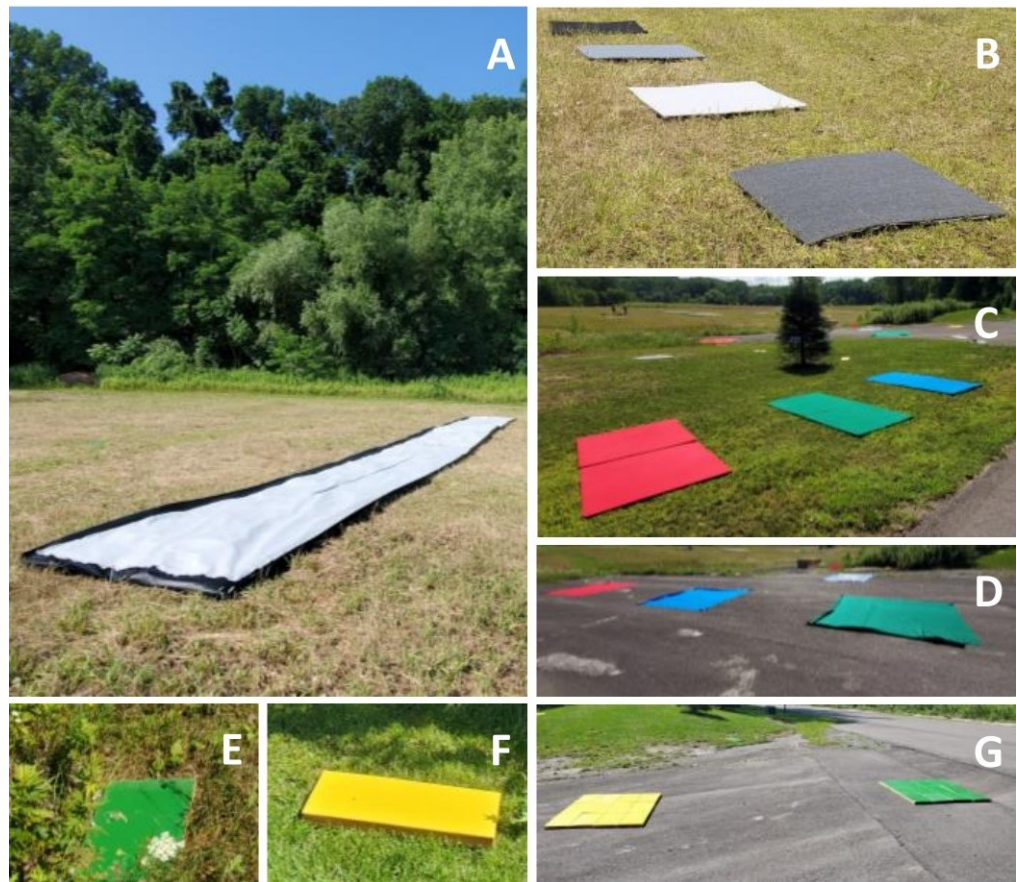
Figure 5. Reflective targets deployed during the G-SCALE included a long, spectrally flat tarp that was used to assess the impact of adjacent trees across the target area (A) and grey-scale felt calibration panels (B), as well as colored diffuse panels and tarps (C,D). In addition to these standards, small green and yellow panels (E,F) were distributed throughout the study area at random orientations and locations for spectral target detection and pixel unmixing studies and as large targets (G) for endmember extraction.
