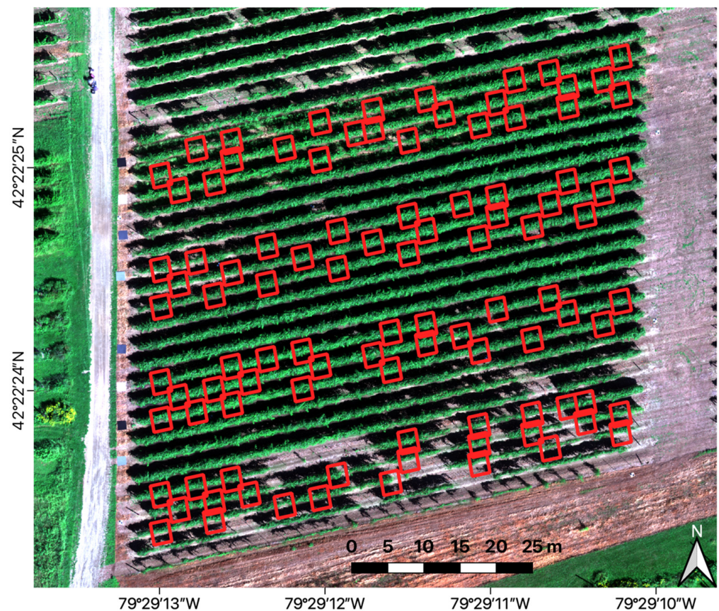
Figure 1. MicaSense Rededge-M 5-band reference imagery (RGB channels shown; see Section 2.2) of the 1-acre Concord grapevine vineyard block located at CLEREL in Portland, NY, USA. The imagery was taken on 6 September 2021 at 10:55 a.m. EST. The 100 vine sampling locations are marked with red squares (2.5 m × 3.0 m).
