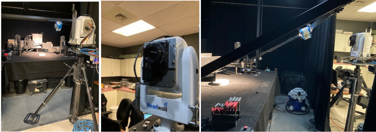
Figure 4. (Left) Experimental Setup from point of view of the hyperspectral imaging system, (middle) the hyperspectral imaging system with the polarizer and rotation stage attached, (right) side view of the experimental configuration.
