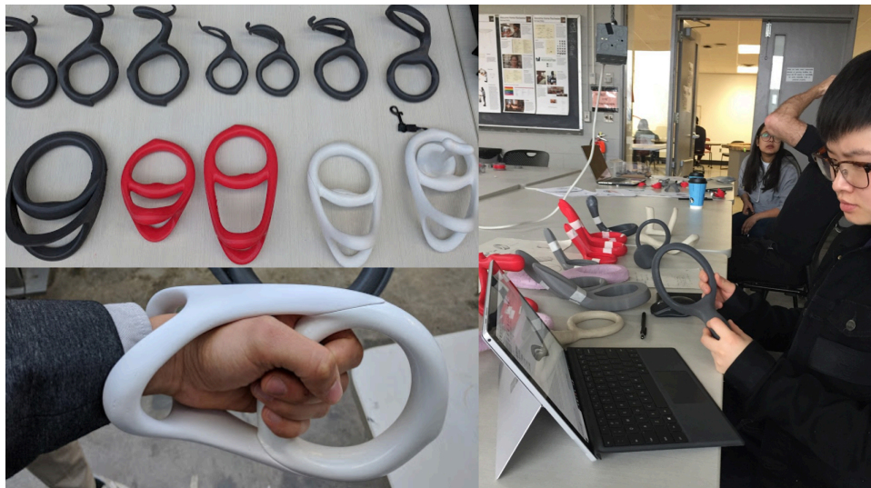
Figure 2: Samples of models from one of the students, including clay, foam, 3D printed, and CAD formats.
