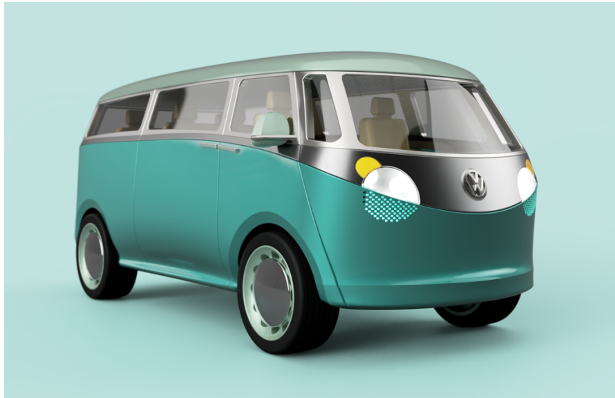
Figure 13: VW van concept. The angle of the light creates interesting gradients in the van's surfaces. The highlights in the wheels, bumpers, side trims and windows provide extra information for understanding the geometry of the design.
