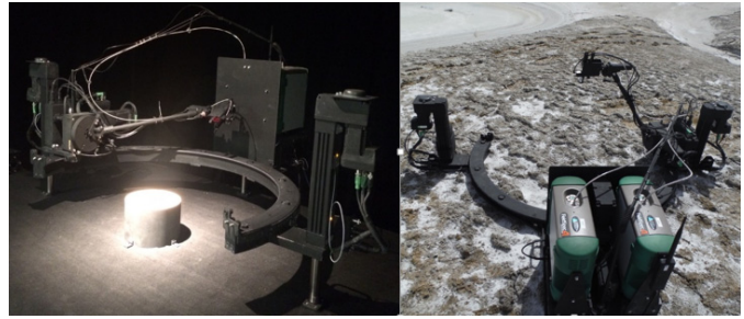
Fig. 1. (Left) GRIT-T in the laboratory setting with sample in holder. (Right) GRIT-T in a field setting.
