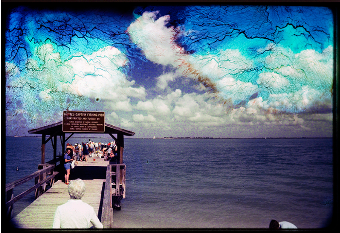
(Above) Florida in March 1981 Kodachrome slide film: top image is before the treatment, bottom image - aged 7 days at 90F at 100% humidity.
