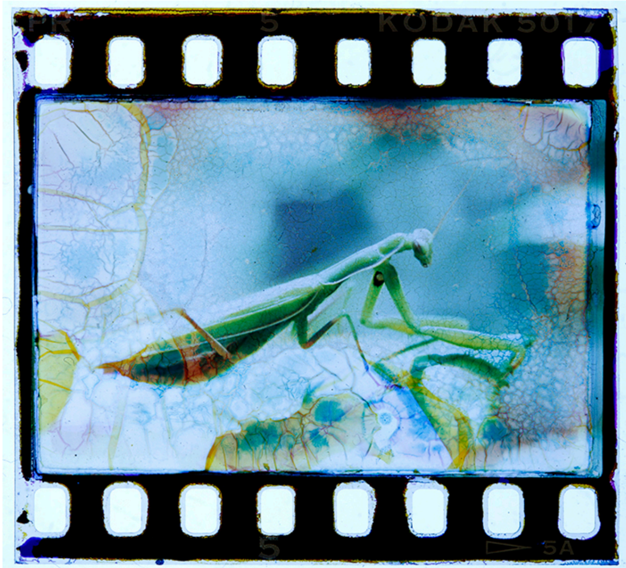
(Above) Kodak Ektachrome Elite 200 slide film 1992: aged 7 days at 90F at 100% humidity.
