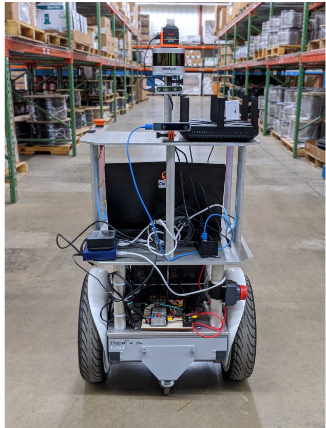
Figure 1. The autonomous platform used to collect localization sensor samples for model training and evaluation. Several sensors including a Kodak PixPro sp360 4K omnidirectional camera (top) and a Velodyne VLP-16 3D LiDAR (below sp360 4K) provide an abundance of features useful for robot localization.
