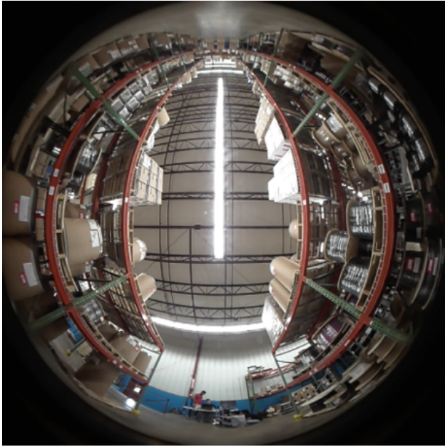
Figure 2. Omnidirectional camera image taken using the Kodak PixPro sp360 inside the warehouse testing environment.
