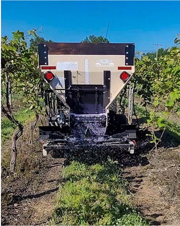
Figure 1. Lanco variable-rate fertilizer spreader in action.
