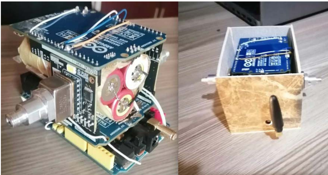
Figure 1: Two views of the prototype for measuring water remote sensing reflectance. Left – The packaged system showing the detail of the fiber optic connector attached to the Hamamatsu mini-spectrometer, with rechargeable batteries and GSM module on the bottom. Right – Packaged system showing the two fiber connectors for the two required measurements, and the GSM module.
