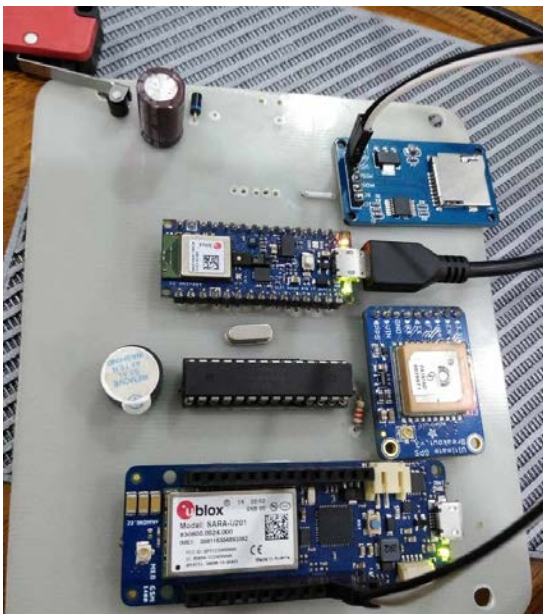
Figure 1: Prototype system for field deployment. This system uses Arduino compatible parts, including the acoustic sensor, GPS for accurate timing, the ability to apply compact machine learning models on the data, and GSM service to send an SMS alarm.
