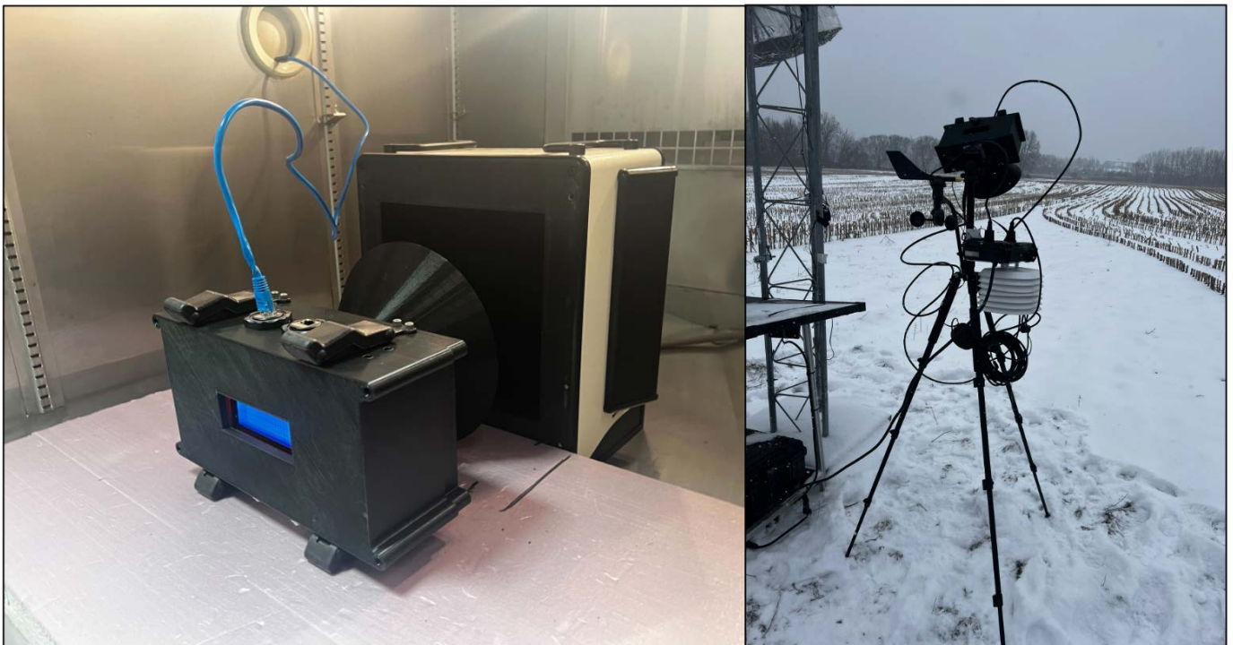
Figure 2: The thermal radiometer developed at RIT for measuring kinetic surface temperature to support Landsat surface temperature product validation. (Left) shows the radiometer being characterized in an environmental chamber and (right) shows the unit integrated with environmental sensors in the field.
