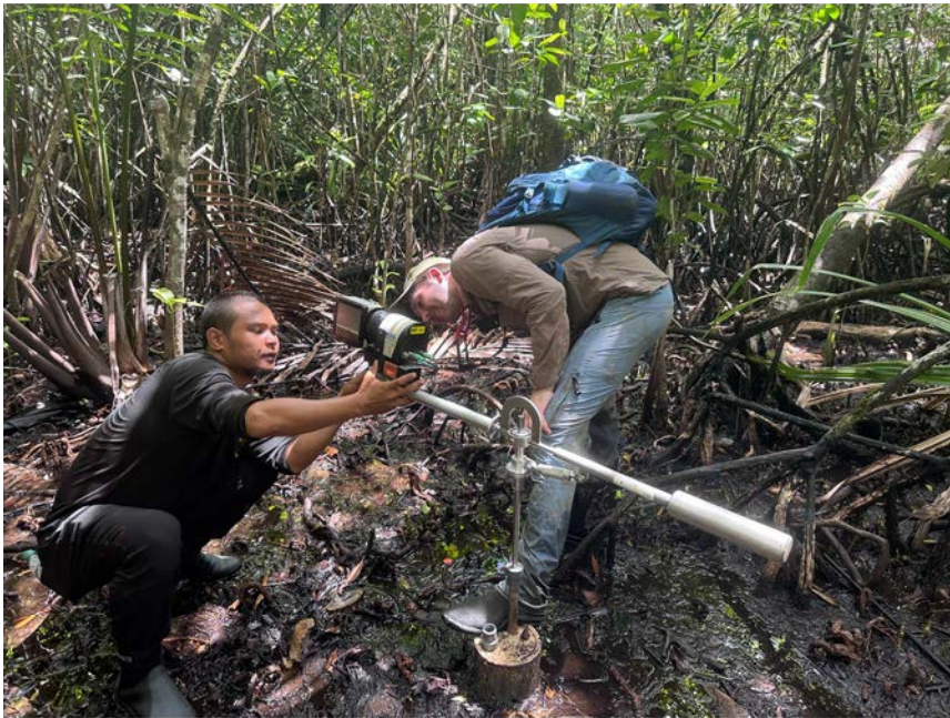
Figure 1. Skyler and Rob setting up the TLS on a surface elevation table.
