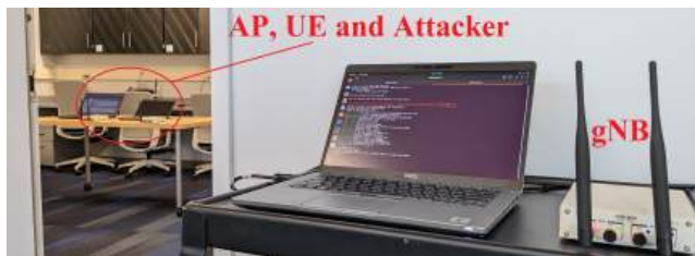
Fig. 15. Complex indoor experimental setup with the AP, UE, and Attacker inside a room and the gNB outside in a hallway.
