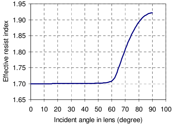
Figure 5. The effective refractive index of the photoresist is a function of the incident angle.
