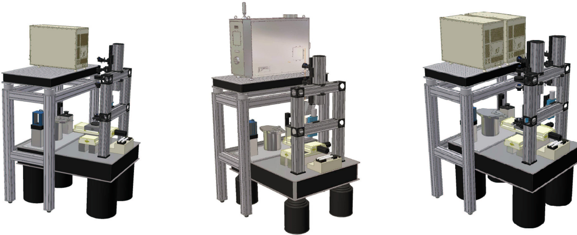
Figure 2. Possible configurations of the Amphibian XIS-SW (left) with OPTEX PRO (center) with BraggStar and (right) with a dual wavelength option.
